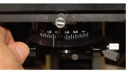
8. Center illumination using the condenser centering screws. Open the field diaphragm some to be sure of position.
