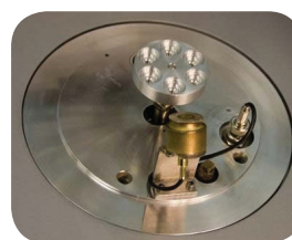
Base plate, standard specimen stage and optional film thickness monitor (FTM)
