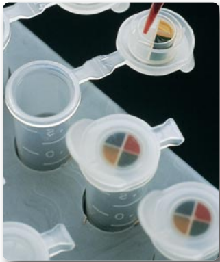
Reaction Vessels Sectors for the 0.5ml tubes hold up to 15µl and sectors for 1.5ml tubes hold 20µl
