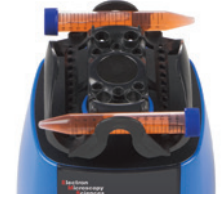
15 mL conical tubes x 2 (horizontally mounted)
