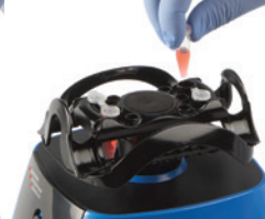
1.5/2 mL microfuge tubes x 4 (vertically mounted)
