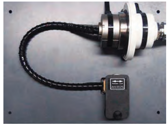
Coolstage and vacuum feed through connected to the storage block (stage protected by plastic shutter)
