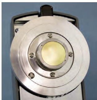
Sputtering insert. Gold (Au) fitted as standard, but other metals available
