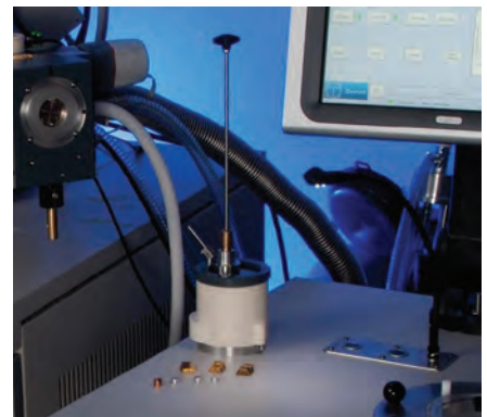
When not in use, the cryo transfer device can be stored under vacuum in the pumped storage tube, located on the Prepdek® work surface
