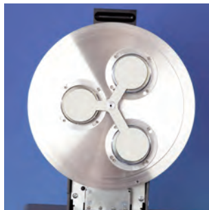
Triple sputtering head with automatic shutter closed
