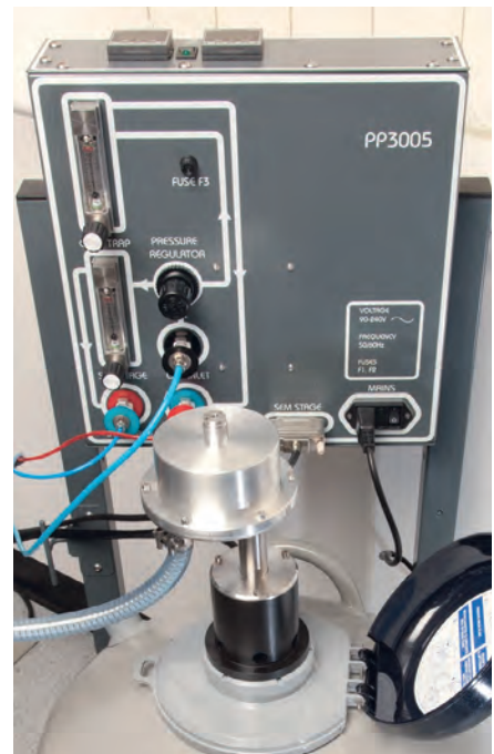
Controller and cooling system
