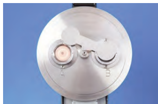
Dual sputtering heads and automatic shutter
