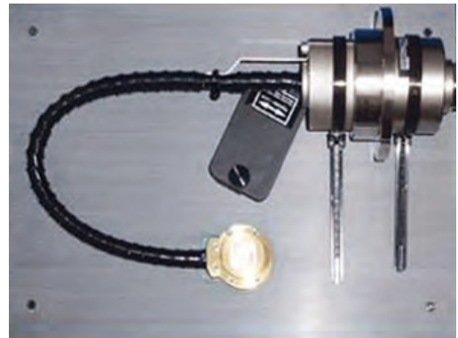
Coolstage and vacuum feed through connected to the storage block (with protection shutter open)
