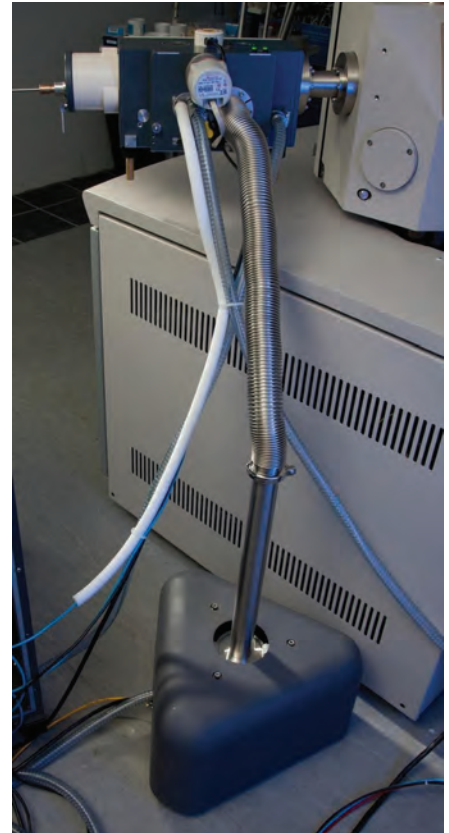
Remotely mounted turbomolecular pumping system
