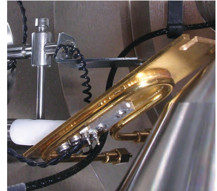
Cold trap - adapted to installation
