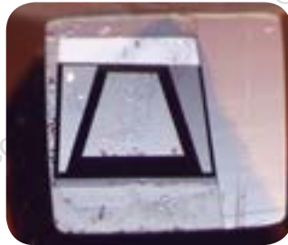
Diamond knife trimmed sample.
