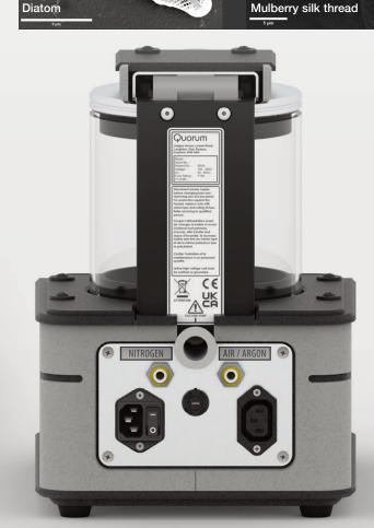
The MiniQS is ideal for the budget-conscious user who also demands reproducible results in an easy-to-use instrument. The MiniQS uses a Magnetron sputtering head with an easily replaceable disc target.
