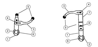
**Figure 3:** Illustration of the 02-02261 Manual Specimen Yoke. On the left is the yoke used for the left side of the Model 910T, and on the right is the yoke used for the right side of the Model 910T.
