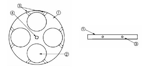
Figure 10: Schematic drawing of Model 92006 fixture. 1- Center hole ; 2- Specimen mounting hole; 3,4- Set screws; 5- Base
