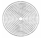
The LP 920MC is a Cast Fe plate machine with concentric grooves in the surface of the plate. These grooves help trap abrasive suspension in them during processing and also reduce the amount of resistance imparted to the specimen during lapping. Large, flat specimens (e.g. 2" (50mm) wafers) are best suited to use on grooved plates to prevent any detrimental effects from friction between the specimen surface and the plate surface.
