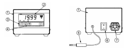
Figure 11: Illustration of the Model 92030 RPM Meter. 1- Main housing; 2- RPM digital display; 3- START button; 4- Range button; 5- Interface cable to Model 910T; 6- MAINS ON/OFF Switch; 7- AC Inlet
