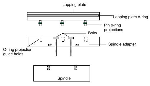
Figure 2: Illustration lapping plate mounting to the Model 910T .
