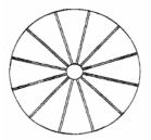
The Model LP 920MR is a Cast Fe plate machined with radial grooves in the surface of the plate. These grooves again help trap abrasive suspension in them during processing and also reduce the amount of resistance imparted to the specimen during lapping. Radial grooves help reduce the possibility of scratching the specimen surface and also improve flatness of the plate during lapping.
