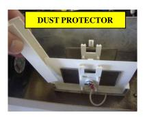
\*NOTE: set dust protectors aside and after you clean the plates inside the machine. Reinstall them by sliding them back onto the slot that they were removed from on the back of the plate holder.
