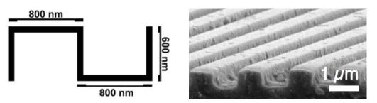
**Figure 1**. *Left*: A schematic showing the approximate dimensions of the nanopattern cross-section. *Right*: A scanning electron micrograph of the nanopattern showing the surface and cross section.
