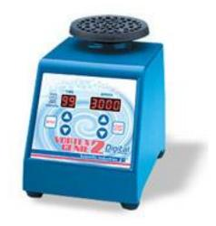
The Digital Vortex-Genie<sup>®</sup>2 is a technologically advanced vortex mixer designed to give the operator true speed feedback. To prevent any confusion, please note that displayed speed is ACTUAL speed, which may differ slightly from SET speed due to load. There is no error with your mixer.
