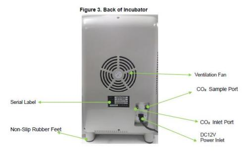
Do not fuse  $CO_2$  inlet port and sample port. Tube from gas cylinder must be connected to  $CO_2$  inlet port. Sample port is used to check the  $CO_2$  density with an external analyzer.
