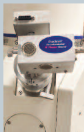
SEM chamber with Evactron De-Contaminator Plasma Radical Source (PRS) attached. An adaptor flange is used to mount the Evactron De-Contaminator to the SEM.
