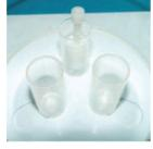
Lynx I specimen vial are locked in and tip-proof during processing. That's the specimen basket it holder assembly in the rear vial.
