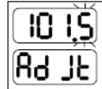
Ex: If the actual read out of thermometer is 39.6, modify the temperature to 39.6 by pressing ▲ or ▼ Then press “Start” to confirm the input value.
