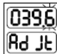
The 40° calibration has now been completed and the dry bath begins the 100°C calibration.
