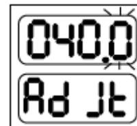
**NOTE:** It is important to allow 20 minutes for the temperature to equilibrate before making any adjustment to the temperature.
