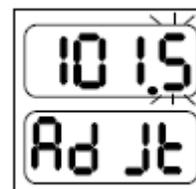
Press “Stop” again (or wait for 6 seconds), then display shows “ **Ad Jt** “. Now adjust the displayed temperature to the measured value (101.5) by pressing ▲ or ▼. Then press the “Start” key to confirm.
