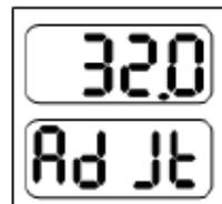
external temperature calibration mode. The temperature displayed is the external probes current temperature and it will begin to rise to 40.0° automatically.
