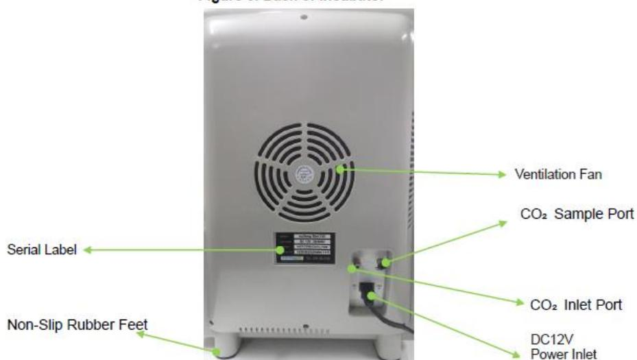
Do not fuse CO<sub>2</sub> inlet port and sample port. Tube from gas cylinder must be connected to CO<sub>2</sub> inlet port. Sample port is used to check the CO<sub>2</sub> density with an external analyzer.
